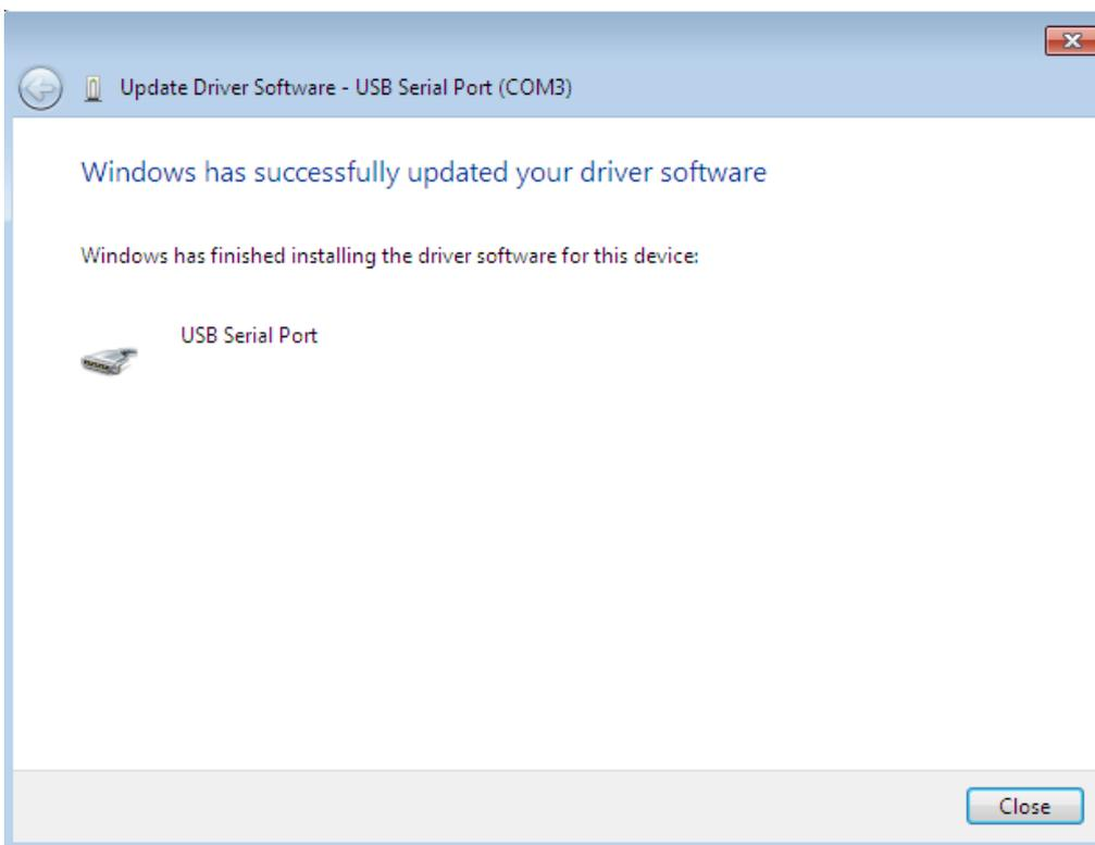
Note this screen also displays the COM port assigned to the device. Press Close to close this window and go back to the Device Manager Window.
