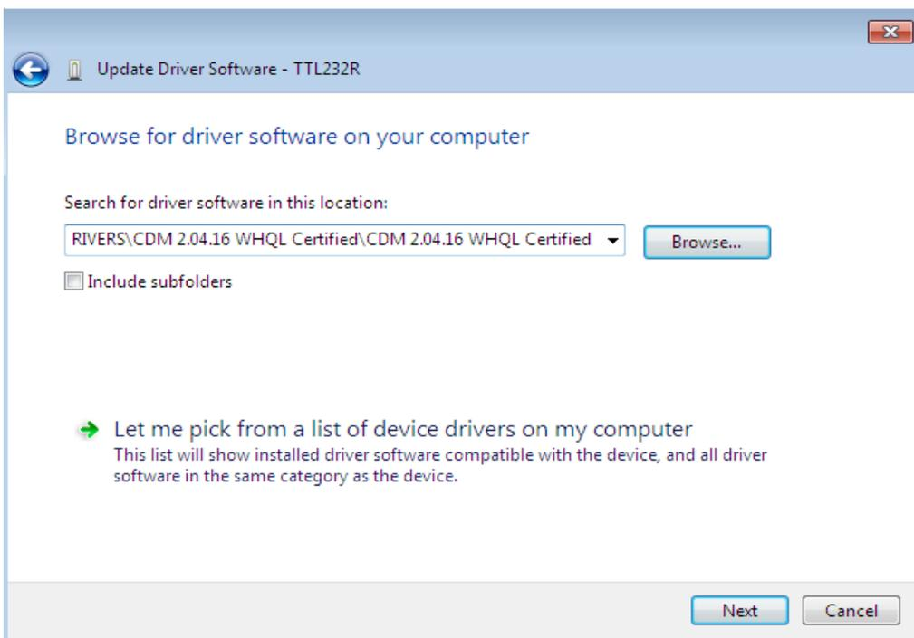
In the address box put the exact location where the drivers have been saved to. This may be in a folder on the PC. It is not necessarily the exact same location as shown in the screenshot. The drivers could have been saved anywhere of the users choosing.
