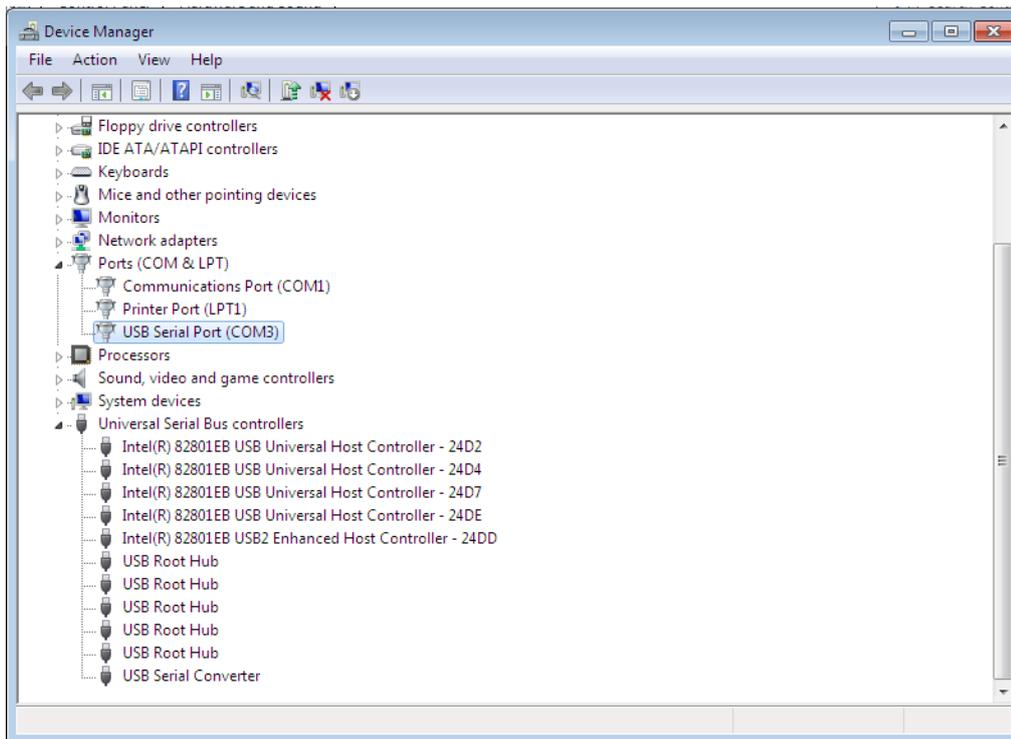
This time the Device Manager does show entries under Universal Serial Bus Controllers and Ports (COM & LPT). The above screen shot displays a correct installation. The device is now ready to use on COM3.
